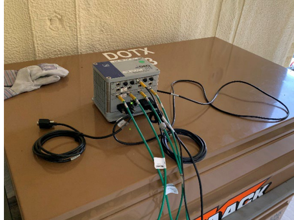
Figure 5. eDAQ Lite Device Setup
