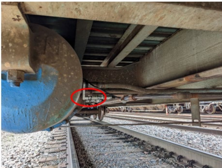
Figure 8. AR and ER Pressure Measurement in Test Car
