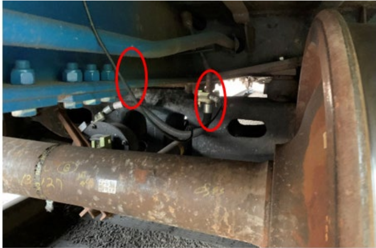
Figure 7. BC Pressure Measurement on Test Car
