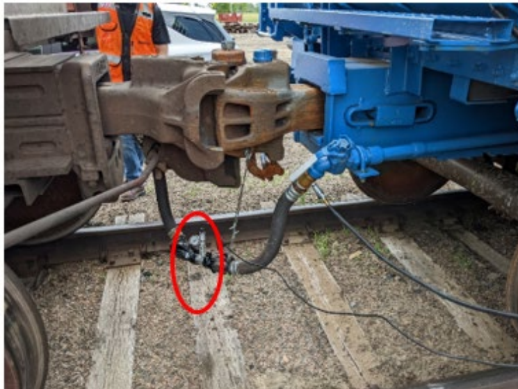
Figure 6. BP Pressure Measurement on Test Car
