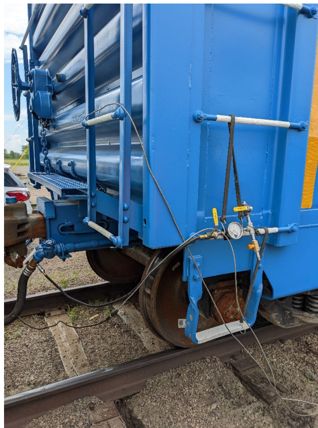
Figure 9. Leakage Port in Test Car
